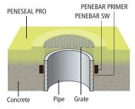
**Drain:** PENEBAR SW waterstop should be installed around the pipe.
