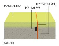
Construction joints: Apply a topical layer of PENETRON crystalline material and/or install PENEBAR SW waterstop between pours.
