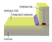
Cold joints: A variety of systems can be used here, including PENEBAR SW waterstop (new construction joints) and PENETRON crystalline topical material (existing construction joints).
