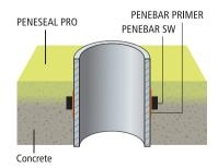
**Penetration:** Install PENEBAR SW waterstop around the penetration.
